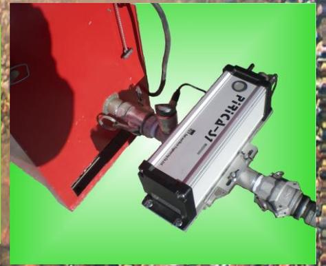
**PIRICA-S1** is the new generation radio-isotope (Nuclear) density meter for piping installation.
